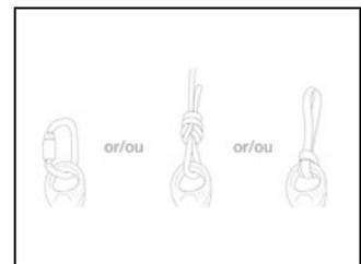
The swivel can be used with ropes and slings for easier rigging and allows most carabiners to rotate, meeting European standards.
